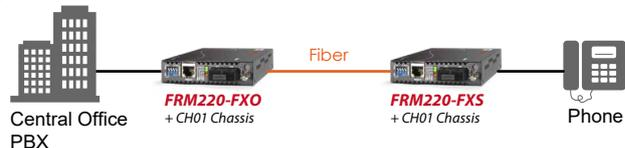
**Figure 3 : Selectable FXO or FXS mode**
