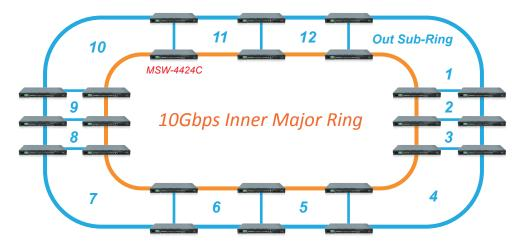
Backbone network extended to the 4G LTE BTS field sites
