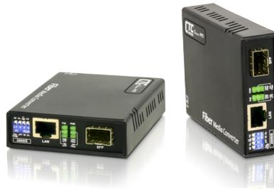
PMC-1000S is a managed Gigabit Ethernet media converter that supports conversion between electrical 10/100/1000Base-T and optical 1000Base-X Ethernet and as PSE (Power Source Equipment) provide PoE+ power over Ethernet. PMC-1000S provides an SFP cage for 100/1000Base-X compatible SFP modules. By offering in-band management, this converter can be remotely controlled and monitored in a centrally located managed rack via FMC-1800 media converter rack.
