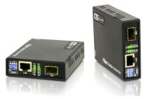
PMC-1000S is an managed Gigabit Ethernet media converter that supports conversion between electrical 10/100/1000Base-T and optical 1000Base-X Ethernet and as PSE (Power Source Equipment) provide PoE+ power over Ethernet. PMC-1000S provides an SFP cage for 100/1000Base-X compatible SFP modules. By offering in-band management, this converter can be remotely controlled and monitored in a centrally located managed rack via FMC-1800 media converter rack.
