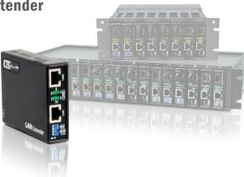
CTC's LAN Extender pair (LX100) can extend data beyond the 100 meters limitation of standard Ethernet. The paired units work in a point-to-point topology over 1 or 2 pair unshielded twisted pair (UTP) cabling up to 800 meters. These products can extend your 10/100Mbps Ethernet network by up to 800m over UTP cable.
