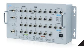
The EN50155 certified managed PoE switch ITP-12164XTM-12PH, that provides 4 10Gigabit, 16 Gigabit M12 X-code Ethernet ports and 12 Megabit M12 D-code, features total 12 ports PoE and supports a variety of PoE operation functions, including automatic detection of PoE device power, automatic reset, PoE scheduling, etc.
