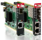
The FRM220A-2000EAS/1 and FRM220A-2000EAS/2 are OAM compliant Gigabit Ethernet switch designed to make conversion between 10/100/1000Base-T(X) + 100/1000Base-X SFP (2000EAS/1) and  $2 \times 10/100/1000Base$ -T(X) +  $2 \times 100/1000Base$ -X SFP (2000EAS/2).
